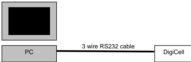
Figure 1. Connection for RS232 port DigiCell devices
